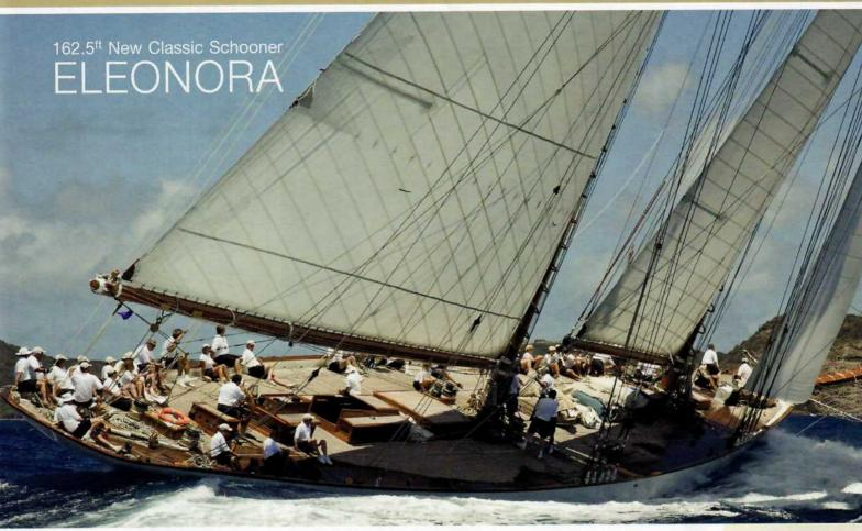
Steel hull with teak superstructure, ELEONORA is an exact replica of the schooner Westward which was designed in 1910 by Nathanael Greene Herreshoff, the 'Wizard of Bristol', the designer of the America's Cup defenders which were undefeated throughout all six challenges from 1893 to 1920. Westward was arguably one of the most famous racing schooners in the world.
